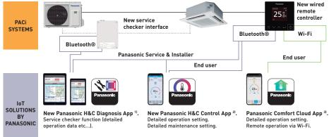
1) A service checker interface is required when this app is used from outdoor location. Wired remote controller (CZ-RTC6BL or CZ-RTC6BLW) is required when this app is used from indoor location. Available from winter 2020, compatible with PZ3 and PZH3 outdoor units. 2) CZ-RTC6BL or CZ-RTC6BLW required. 3C -RTC6BLW required. 3C -RTC6BLW required. 3C -RTC6BLW required.
