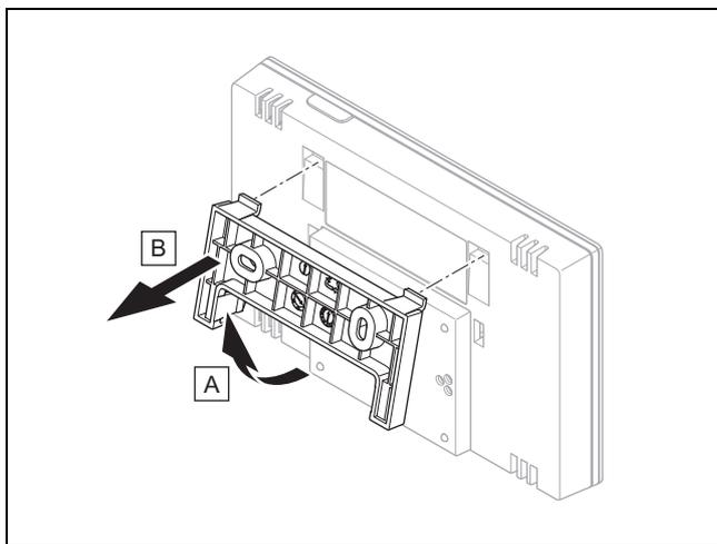
6. Remove the unit mounting bracket from the system control as shown in the figure.
