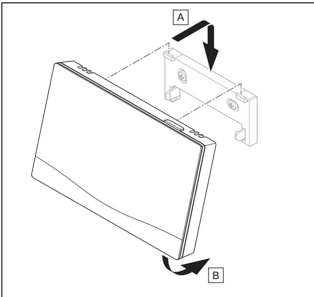
7. Clip the system control into the unit mounting bracket as shown in the figure, making sure that it clicks into place.
