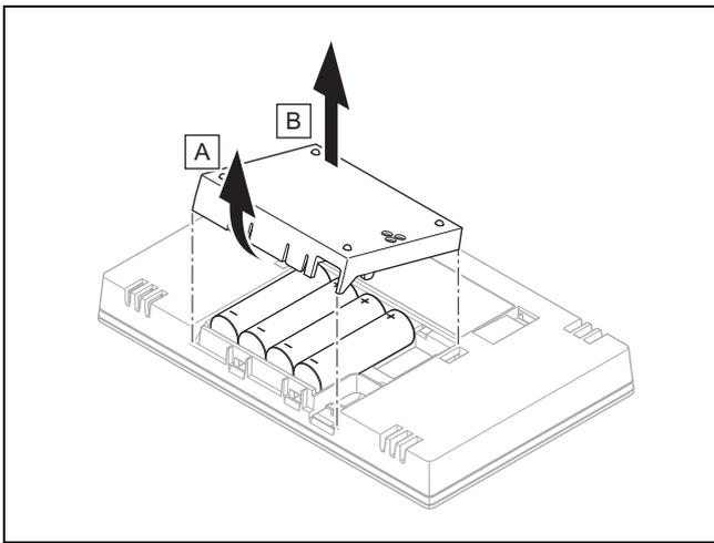
4. Open the system control's battery compartment as shown in the figure.
