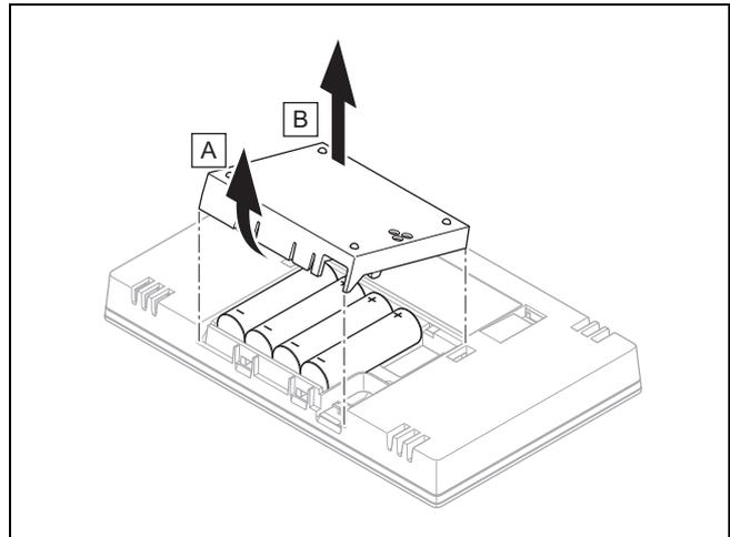
2. Open the battery compartment as shown in the figure.
