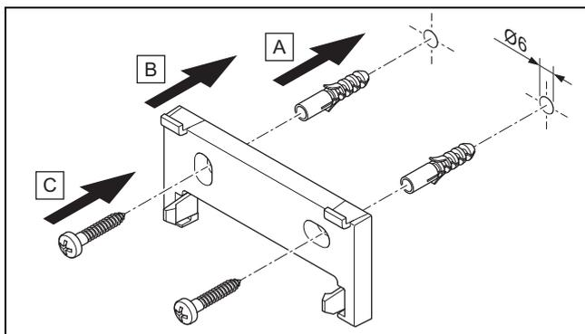
7. Secure the unit mounting bracket in accordance with the figure.
