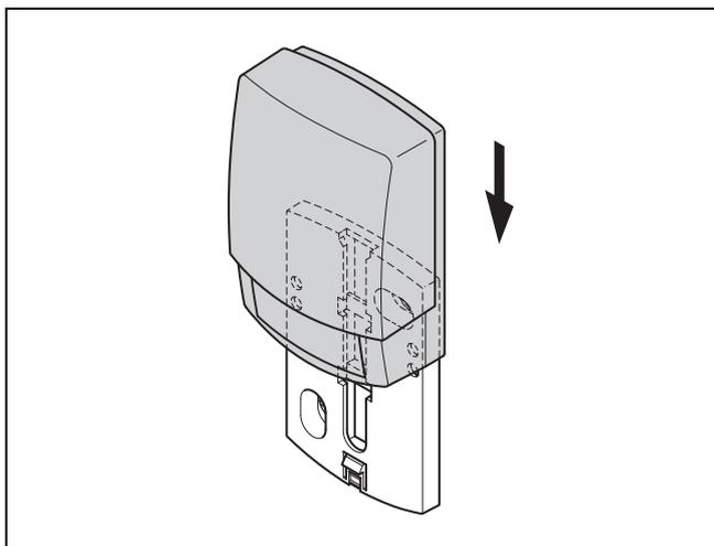
2. Fit the outdoor temperature sensor to the wall base as shown in the figure.
