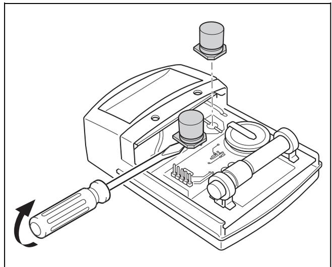
2. Remove the capacitors as shown in the figure.
