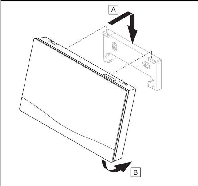
8. Fit the system control to the unit mounting bracket as shown in the figure, making sure that it clicks into place.
