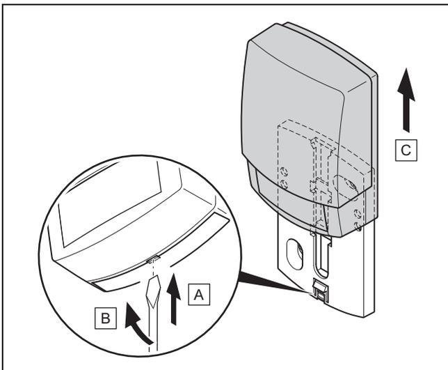
1. Remove the outdoor temperature sensor from the wall base as shown in the figure.
