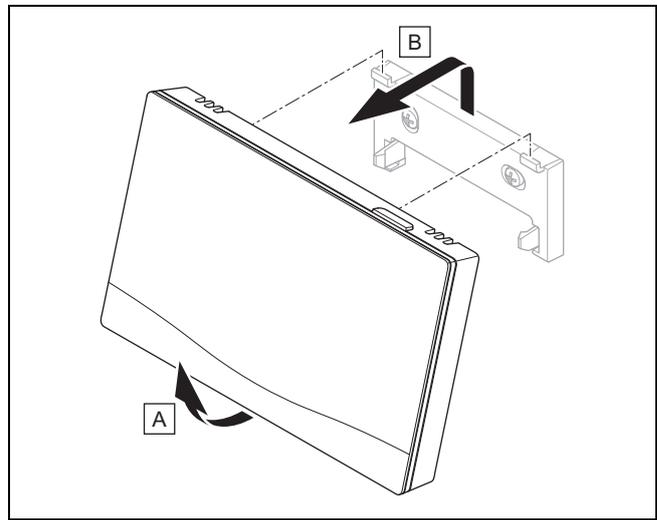
1. Remove the system control from the unit mounting bracket as shown in the figure.
